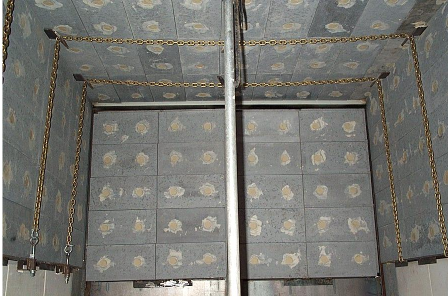
Refractory lined burn chamber
